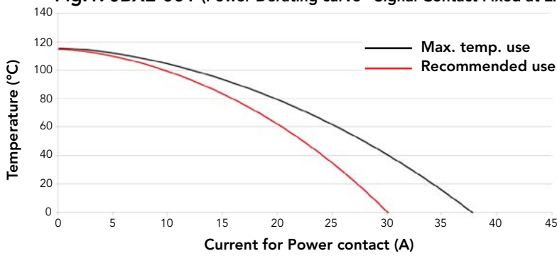
Fig.1: JBX2-001 (Power Derating curve - Signal Contact Fixed at 2A)
